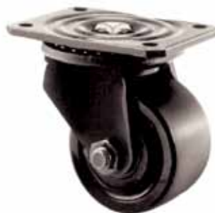
SLP14-RTR-3 & SLP14H RTR-3 3" wheel Capacity to 1200 lbs Top Plate: 3 5/16 x 4 5/16 Mounting: 2 3/8 x 3 3/8 Options: 1, 2, 4, 5
