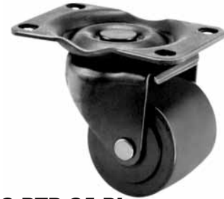
SLP2-RTR-25-BL 2" or 2 1/2" wheel Capacity to 400 lbs Top plate: 2 9/16 x 3 5/8 Mounting: 1 3/4 x 2 7/8 - 3 Options: 1, 2
