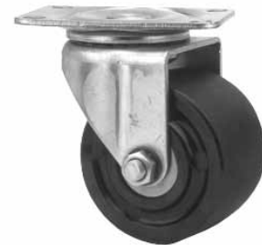
SLP4X-RTR-3 3" wheel capacity to 700 lbs Top plate: 2 5/8 x 3 1/2 Mounting: 1 3/4 x 2 7/8 - 3 Options: 2, 3, 4
